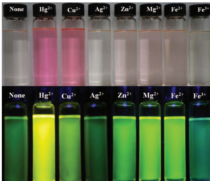
Figure 1. Photo images for absorption color (top) and fluorescence emission color changes (bottom) from the complex of dye sensor 1 ( 10\ \mu\text{M} ) and metal ions ( 10\ \mu\text{M} ) in \text{CHCl}_3:\text{THF} ( v/v 9:1) such as none, \text{Hg}^{2+} , \text{Cu}^{2+} , \text{Ag}^{2+} , \text{Zn}^{2+} , \text{Mg}^{2+} , \text{Fe}^{2+} and \text{Fe}^{3+} (from left to right).
